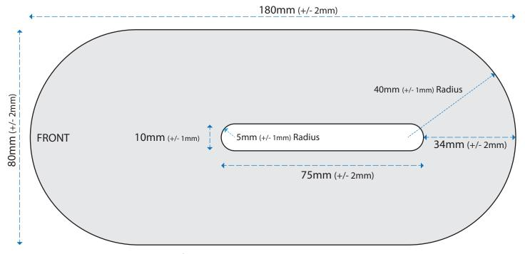
Diagram 1 Keelbox Sticker. (Note: This diagram is full size and can be used as a template if printed at 100%)
